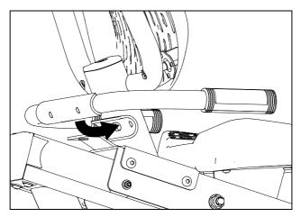
Figure 9: Positioning the handlebars
